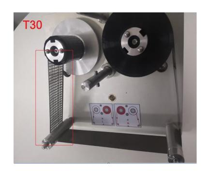
Ribbon rolling is controlled by dual electric motors to keep rolling stable.
