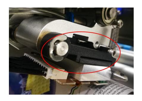
Print head of W30+/W50+ can be repositioned easily by parameter adjustment, and printing angle can be self adapting to different cushion or rubber rolls to ensure printing quality.
